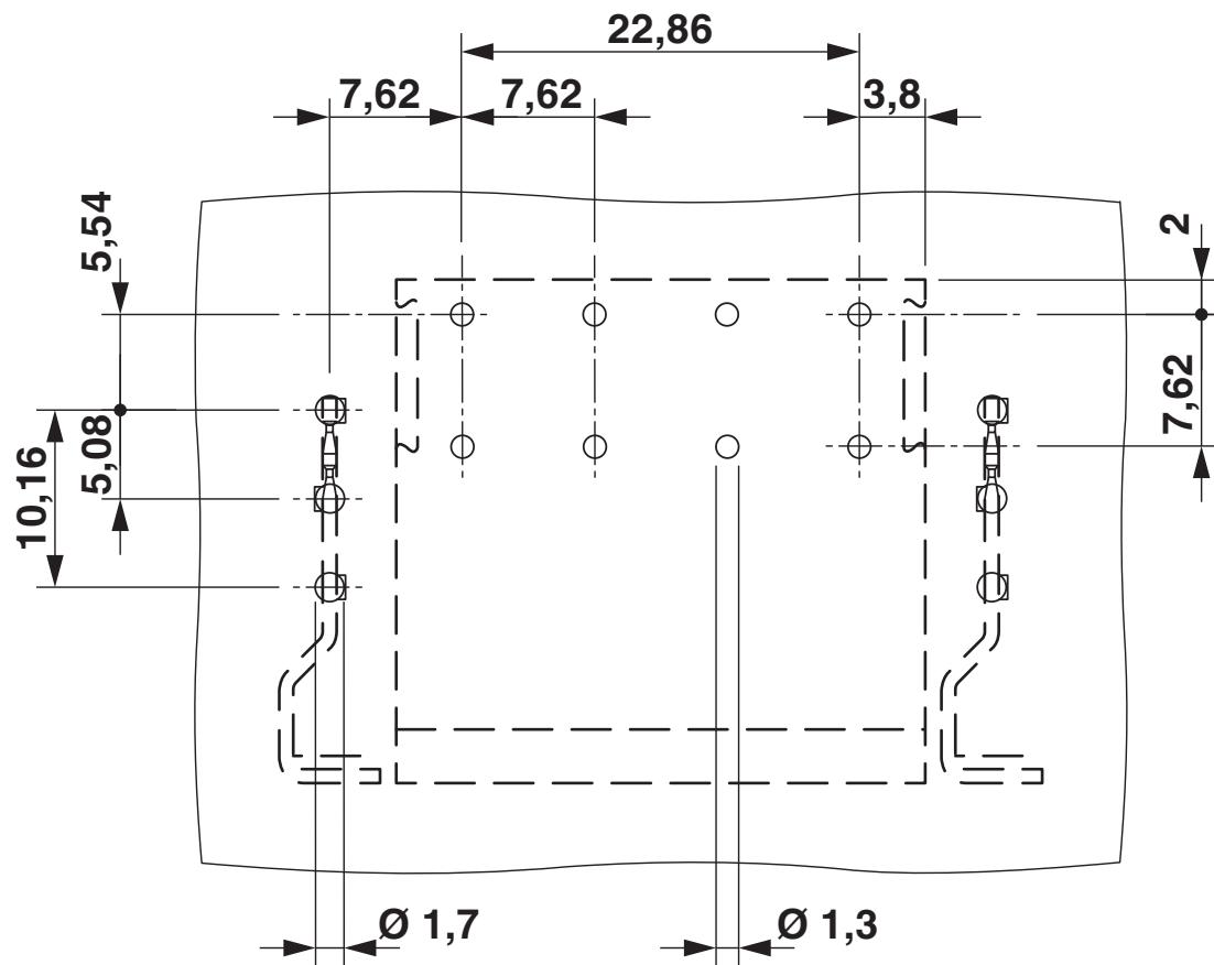
The figure shows the product in conjunction with the POWER COMBICON header PC 4/4-G-7,62
