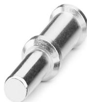
Crimp contact, series: HC-M-...-35, Pin, turned, contact diameter: 8 mm, connection cross section: 25 mm<sup>2</sup> ... 25 mm<sup>2</sup>, AWG 4...4, contact material: Cu alloy
