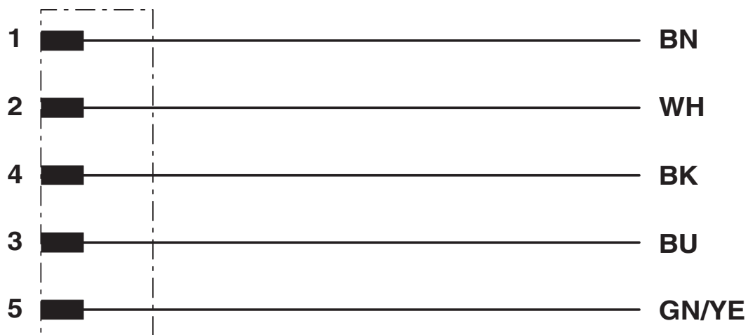
Contact assignment of the M12 plug
