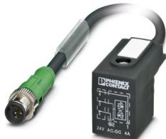
Sensor/actuator cable, 3-position, PUR halogen-free, black-gray RAL 7021, Plug straight M12, coding: A, on Valve connector BI (11 mm), Wiring: Z diode, cable length: 3 m
