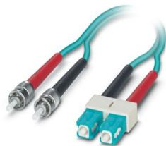
Assembled FO cable, zip cord cable, multimode fiberglass 50/125 µm, OM3, plug: SC duplex/B-FOC (ST), degree of protection: IP20, for installation in cable ducts or control cabinets, length: 2 m
