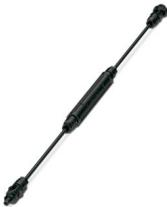
Fuse plug, Range of articles: SUNCLIX, color: black, rated voltage: 1500 V DC (bis 4000m ü. NN), rated current: 11 A, Connection method: SUNCLIX PV connector, SUNCLIX fuse element for protecting panels and devices in photovoltaic systems
