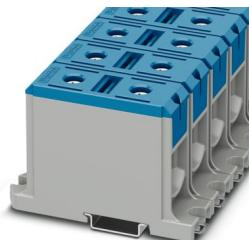
High-current terminal block, nom. voltage: 1000 V, nominal current: 290 A, number of connections: 2, number of positions: 1, connection method: Screw connection, Rated cross section: 150 mm<sup>2</sup>, cross section: 35 mm<sup>2</sup> - 150 mm<sup>2</sup>, Rated cross section: 150 mm<sup>2</sup>, cross section: 35 mm<sup>2</sup> - 150 mm<sup>2</sup>, mounting type: NS 35/15, NS 35/7,5, color: blue
