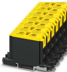
High-current terminal block, nom. voltage: 1000 V, nominal current: 145 A, number of connections: 2, number of positions: 1, connection method: Screw connection, Rated cross section: 50 mm<sup>2</sup>, cross section: 6 mm<sup>2</sup> - 50 mm<sup>2</sup>, Rated cross section: 50 mm<sup>2</sup>, cross section: 4 mm<sup>2</sup> - 50 mm<sup>2</sup>, mounting type: NS 35/15, NS 35/7,5, color: yellow
