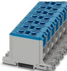
High-current terminal block, nom. voltage: 1000 V, nominal current: 145 A, number of connections: 2, number of positions: 1, connection method: Screw connection, Rated cross section: 50 mm<sup>2</sup>, cross section: 6 mm<sup>2</sup> - 50 mm<sup>2</sup>, Rated cross section: 50 mm<sup>2</sup>, cross section: 4 mm<sup>2</sup> - 50 mm<sup>2</sup>, mounting type: NS 35/15, NS 35/7,5, color: blue
