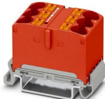
Distribution block, Block with horizontal alignment, nom. voltage: 800 V, nominal current: 57 A, number of connections: 6, connection method: Push-in connection, Rated cross section: 10 mm<sup>2</sup>, cross section: 0.5 mm<sup>2</sup> - 16 mm<sup>2</sup>, mounting type: NS 35/7,5, NS 35/15, color: red
