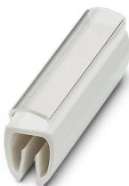
Conductor marker carrier, transparent, unmarked, cable diameter range: 2.8 ... 4.4 mm, mounting type: clip on, text field height: 4 mm, text field width: 12 mm
