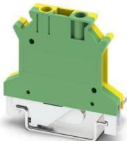
Protective conductor terminal block, number of connections: 2, number of positions: 1, connection method: Screw connection, cross section: 0.2 mm<sup>2</sup> - 4 mm<sup>2</sup>, mounting method: PE foot with mounting screw, M3, mounting type: NS 35/7,5, NS 35/15, NS 32, color: green-yellow
