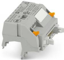
V8 adapter for 8 x PLC-INTERFACE (6.2 mm), controller: PLC system cabling of input cards, connection 1: IDC/FLK pin strip 1x 14-position, connection 2: Plug-in connection (Can be snapped onto 8x PLC-INTERFACE terminals), connection 3: Screw connection 1x 2-position, number of channels: 8, control logic: minusschaltend
