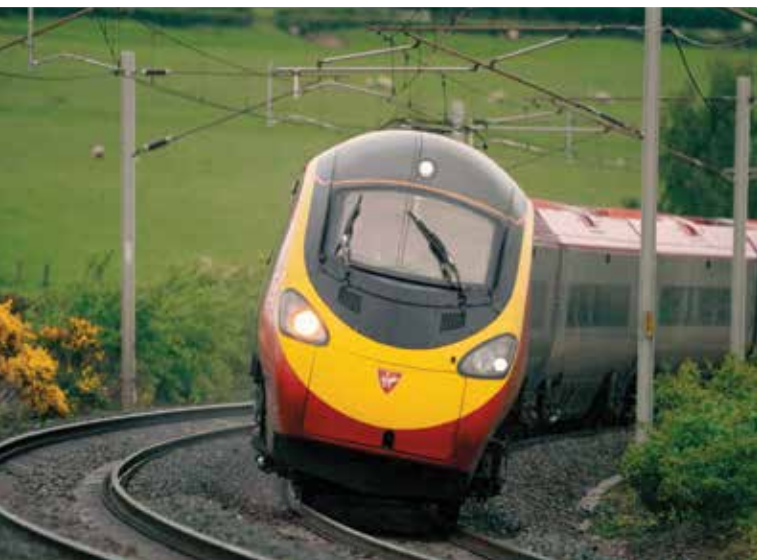
Pendolino (from the Italian Pendolo) is an Italian family of tilting trains manufactured by Fiat Ferroviaria
