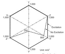
Sample: G5Q-1A-EL-HA-VH Number of Relays: 5 pcs Test conditions: Measure the value of contact malfunction happening by applying 3 axes with 6 direction 3 times each.
