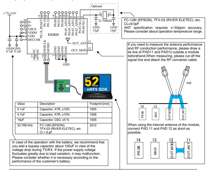
SWD (Serial Wire Debug) is a high performance 2-pin debug port that replaces JTAG. You can debug and program with J-link etc. When using J-LINK, it is convenient to mount a socket on the customer's main board. The socket will be 10-pin connector two rows of 1.27mm pitch (Ex: PSS-720153-05, Hirosugi instrument). J-Link Lite operates at 3.3 V. do not operate at 1.8 V, so please be careful.
