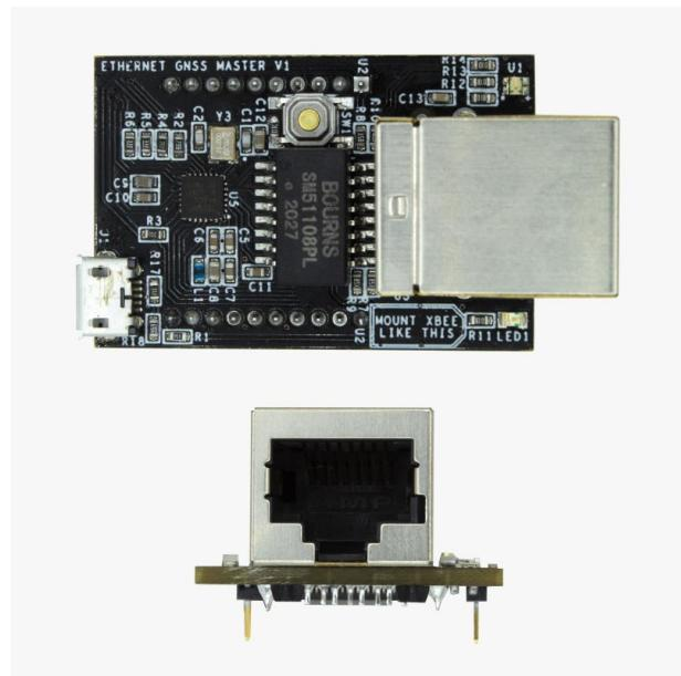
Ethernet NTRIP Master SKU is: AS-XBEE-ETH-100-RJ45-00
