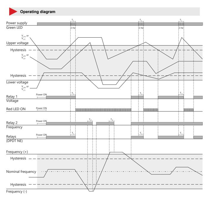
Over / under voltage and over / under frequency monitoring (2 x SPDT relays)
