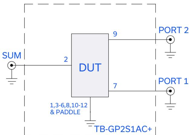
Figure 2. GP2S1A+ Characterization and Application Circuit.
