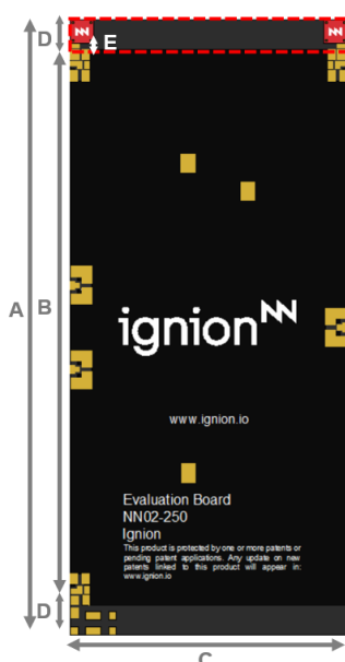
Figure 1 – EB_NN02-250-UFL2R. Evaluation Board with UFL cables. From 824 MHz to 960 MHz and from 1710 MHz to 2690 MHz.
