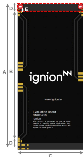
Figure 5 – EB_NN02-250-CPW2R. Evaluation Board with coplanar grounded transmission lines. From 824 MHz to 960 MHz and from 1710 MHz to 2690 MHz.
