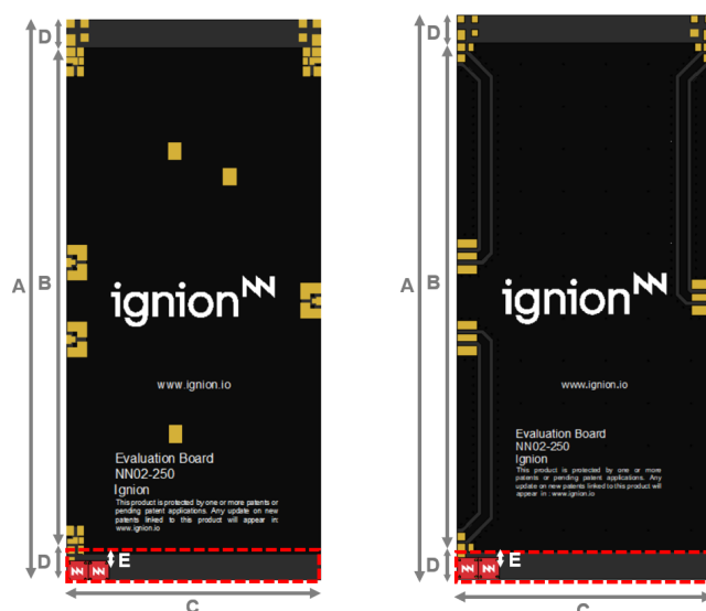
Figure 1 – Evaluation Boards providing operation at LTE700, 1 port configuration.
