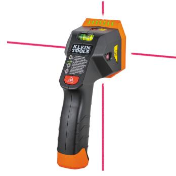
Electronic Stud Finder with Cross-Line Lasers detects hidden wood and metal studs with an auto deep scan of up to 1-1/2-Inch. The horizontal and vertical lasers can be used together or independently. Offering mutable audible alerts and bright LEDs across the top, it clearly indicates the full width of the stud. It features an ergonomic handheld grip, hold mode and withstands a 6.6-Foot (2 m) drop. Felt pads protect walls during use and bubble vial assists with alignment. Laser Class 3R; ?5mW.
