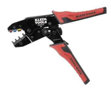
The full-cycle Ratcheting Crimper crimps 10-22 AWG heat shrink wire terminals. This tool features three crimping cavities in one tool with color-coded wire markings for three size ranges of heat shrink terminals. Crimper design provides low effort to crimp while maintaining a high terminal pull-off force. Built-in ratchet ensures full-cycle crimping for a uniform crimp every time.
