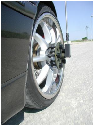
Figure 3: WSS2 wheel speed sensor from PEGASEM Messtechnik GmbH. WSS2 provides wheel tick and direction signals.
