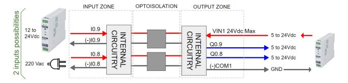
This is a representation of the functioning of this Optoisolated input module. The module is composed of 3 parts: The input zone, the optoisolation and the output zone.
