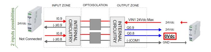
Now we are seeing that the AC supply on the input Io.8 is not present. This means that the input Io.8 is detecting a LOW value. However Io.9 is getting supplied as in all the examples, so it is getting a HIGH value. We can see now that although the VIN1 is getting
