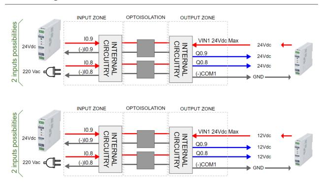
As you can see in these two representations, the voltage established on the VIN1 will be the one that will get the Qo.9 & Qo.8 outputs. The module can provide up to 5 different voltages in pairs of 2 outputs.
