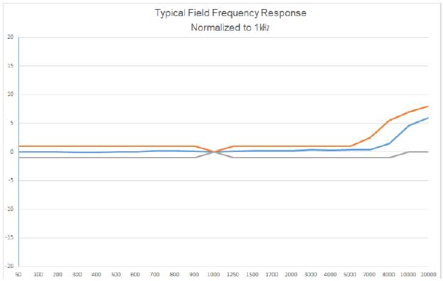
TEST CONDITIONS: 23±2°C, 65±20% R.H., Typical specifications are measured at VDD = 1.8V Speaker: 1Pa(94dBSPL@1kt) at 50cmdistance from a loudspeaker
