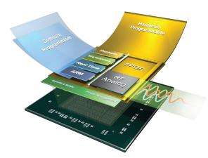
With 200 Gbps of digital I/O available on the FPGA side of the RFSoC, the card supports twice the bandwidth of RFSoC implementations that depend upon PCIe for data transfer. This I/O is available through two QSFP28 ports. Customers have implemented transports using Aurora, Ethernet MAC frames, and UDP.
