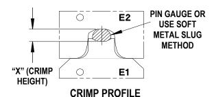
Use gauge pins or soft metal slug (solder) method to measure the "X" dimension. Verify tooling crimp height calibration by referring to the Go/No Go dimensions shown in the chart below.
