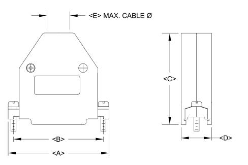
MATERIAL: ABS PLASTIC, UL 94HB RECOMMENDED OPERATING TEMPERATURE: -20°C TO +80°C
