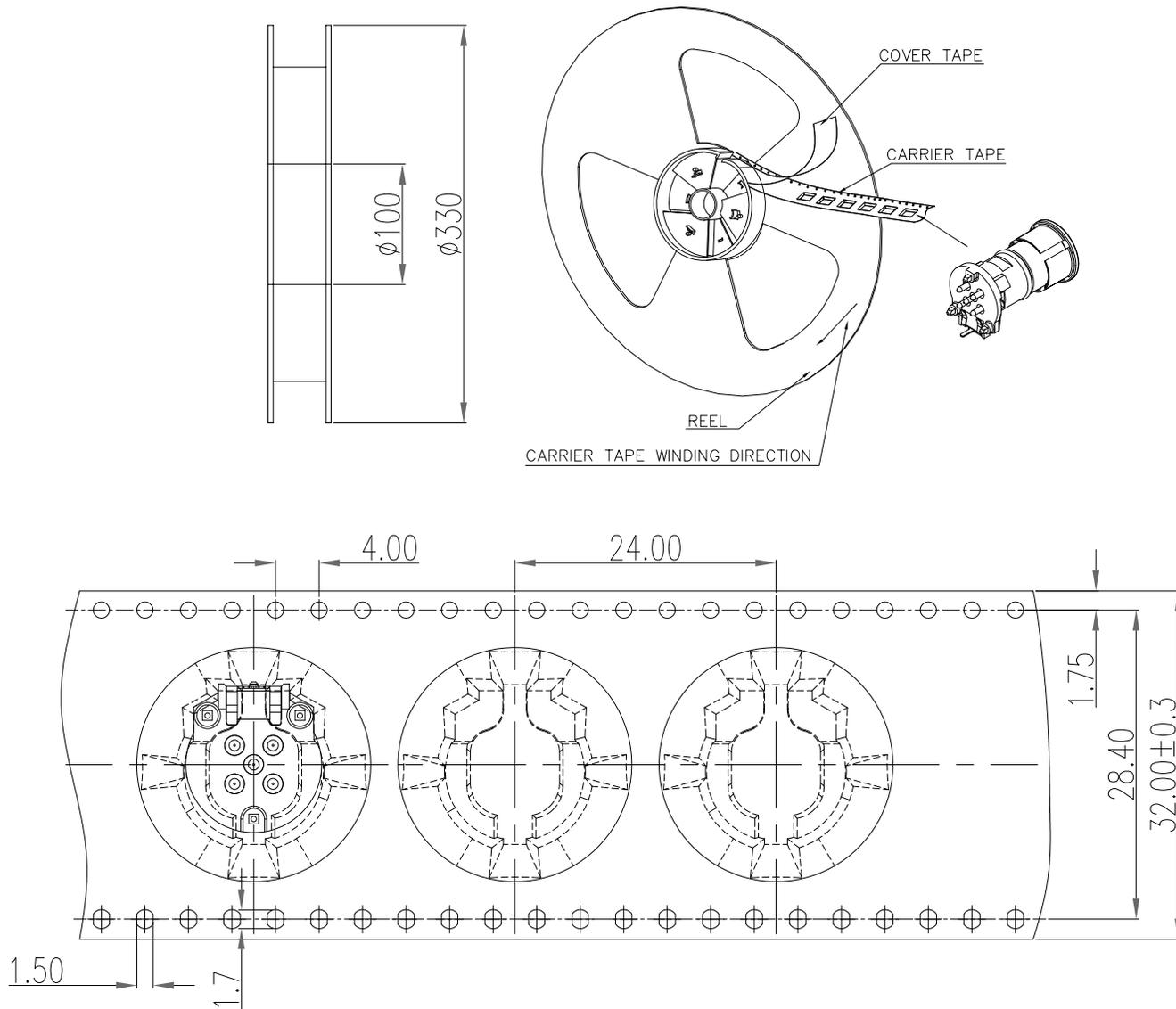
The tape size complies with the (EIA-481-D) specification requirements.
