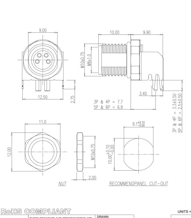
NOTE: MATERIAL HOUSING: PA66 UL94V-0, BLACK CONTACT: BRASS NUT: BRASS SHELL: BRASS ORING: NBR GROUND: PHOSPHOR BRONZE FINISH CONTACT: 10u" GOLD PLATED OVER NICKEL NUT: NICKEL SHELL: NICKEL GROUND: BRIGHT TIN ELECTRICAL RATED CURRENT: 1.5A(5/6P) / 3A(3/4P) 30V(5/6P) / 60V(3/4P) RATED VOLTAGE: 100 MOhms MIN. INSULATION RESISTANCE: CONTACT RESISTANCE: 10 mOhms MAX.
