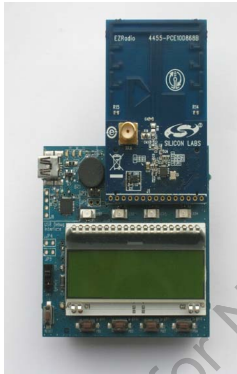
Figure 3. LCD Baseboard with Connected RF Pico Board
