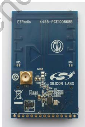
Figure 2. Si4455 RF Pico Board—868 MHz (P/N 4455-PCE10D868B)
