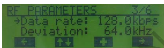
Figure 8. Menu Page: RF Parameters 3/6 (Modulation is 2GFSK)
