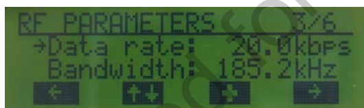
Figure 9. Menu Page: RF Parameters 3/6 (Modulation is OOK)
