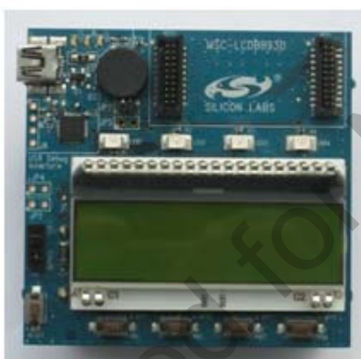
Figure 1. LCD Baseboard (P/N MSC-LCDBB930-PER)
