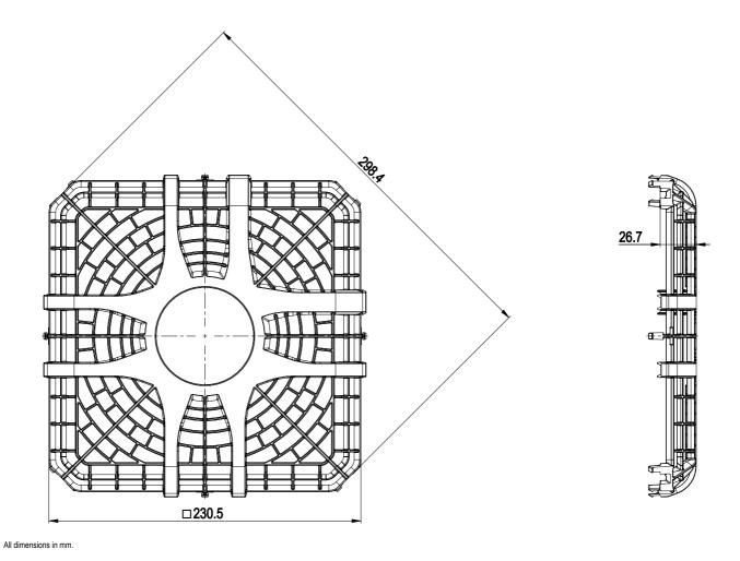
Accessory part: Guard grill 25001-2-2929 on outlet side, not included in scope of delivery
