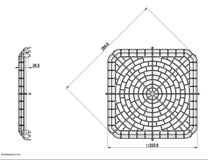
Accessory part: Guard grill 25000-2-2929 on intake side, not included in scope of delivery
