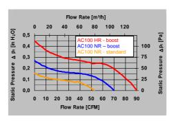
The diagram shows the measured air flow rates of the two standard versions AC 100 NR and AC 100 HR at the standard and boost speeds.
