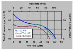
The diagram shows the best of the measured competitive models. The AC 100 NR is slightly superior to the best model. In the speed version H with 4500 min<sup>-1</sup>, the fan performance is considerably higher.
