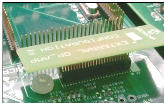
FIGURE 2: EXTERNAL OP AMP CONFIGURATION BOARD
