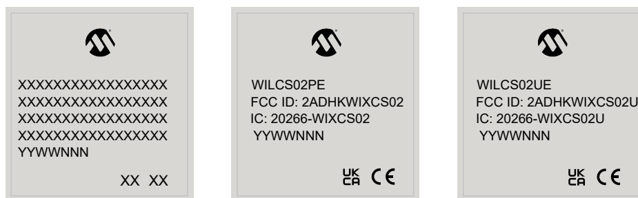
Figure 4-2. WILCS02 Module Packaging Marking
