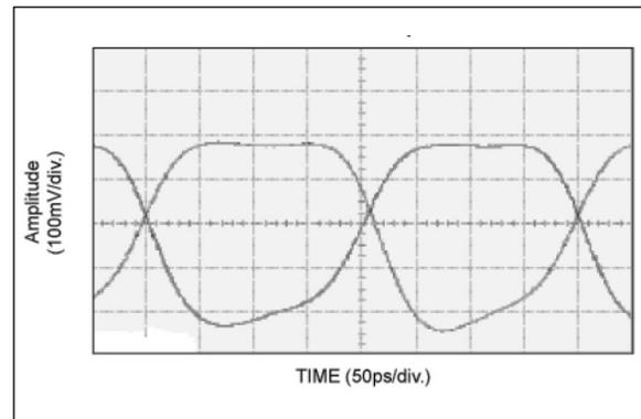
**FIGURE 2-6:** 2.5 GHz Output.
