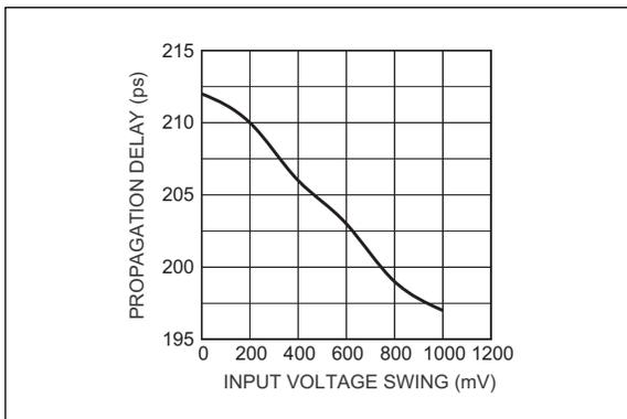
**FIGURE 2-3:** Propagation Delay vs. Input Voltage Swing.
