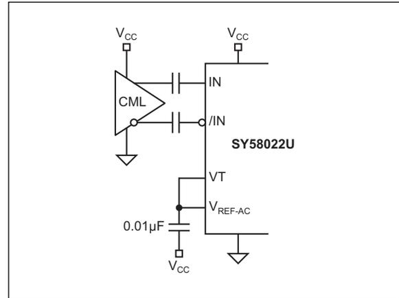
**FIGURE 7-4:** AC-Coupled CML Input Interface.
