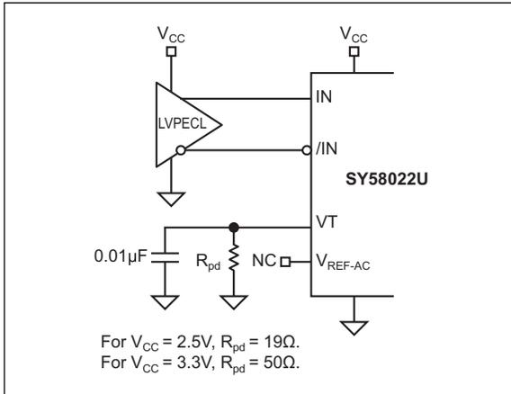
**FIGURE 7-1:** DC-Coupled LVPECL Input Interface.
