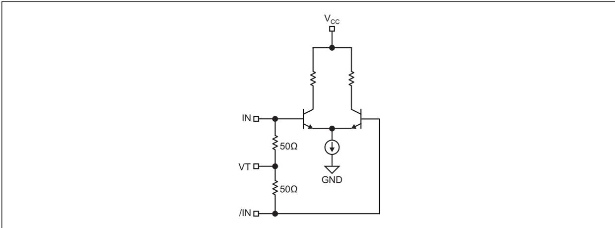
**FIGURE 6-1:** Simplified Differential Input Stage.
