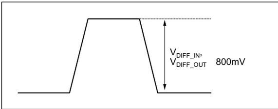
**FIGURE 4-2:** *Differential Voltage Swing.*
