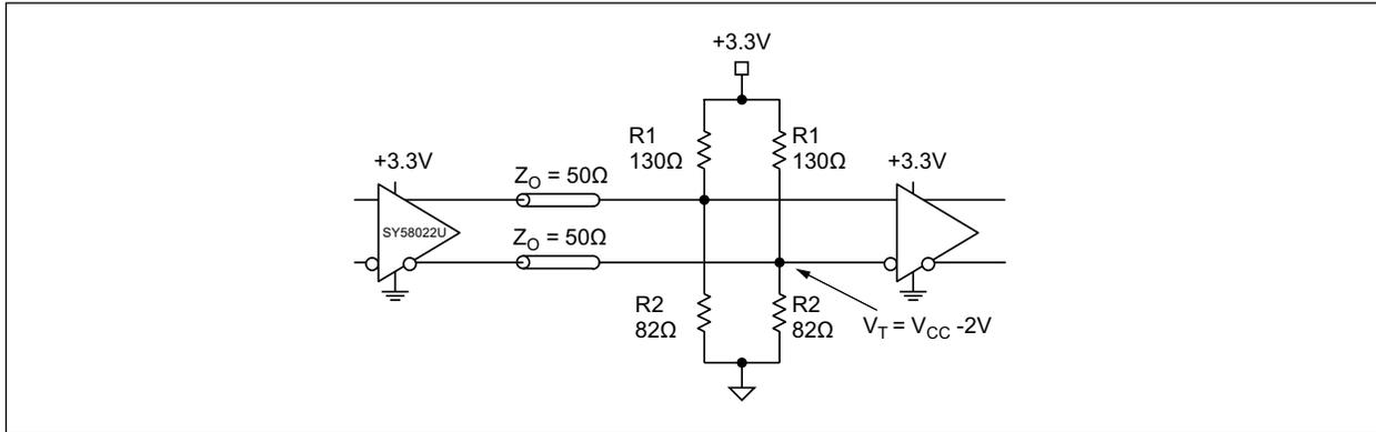
**FIGURE 8-1:** Parallel Termination – Thevenin Equivalent.
