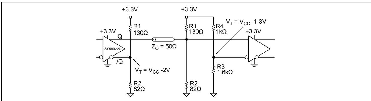
**FIGURE 8-3:** Terminating Unused I/O.
