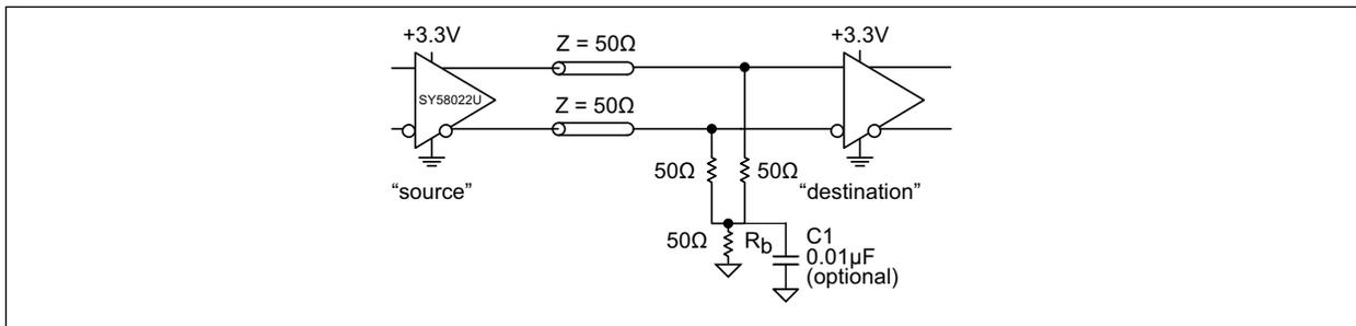
**FIGURE 8-2:** Three-Resistor “Y-Termination”.
