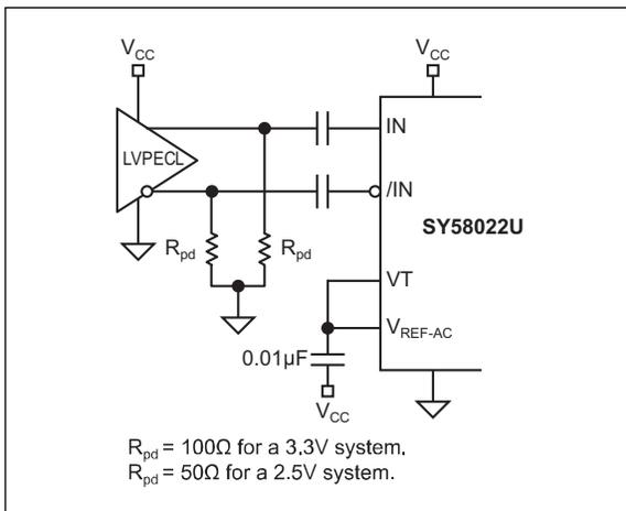
**FIGURE 7-2:** AC-Coupled LVPECL Input Interface.
