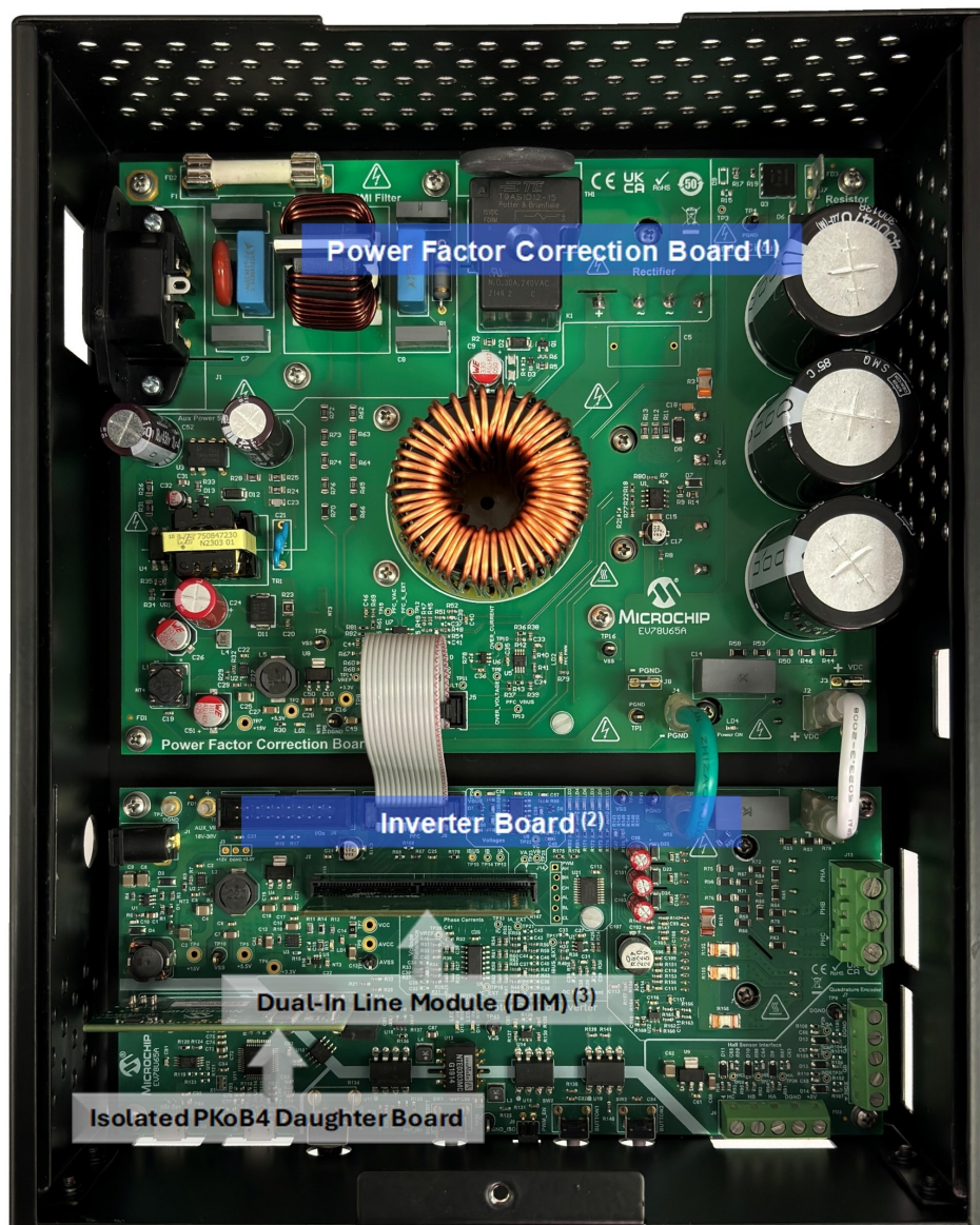
Figure 1. Subcomponents of MCHV-230VAC-1.5kW Development Board
