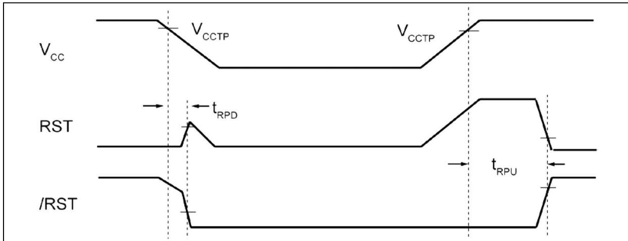
**FIGURE 1-1:** Power-Up/Power-Down Sequence.
