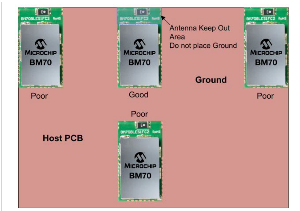
FIGURE 4-3: BM70BLES1FC2 ANTENNA PLACEMENT EXAMPLES
