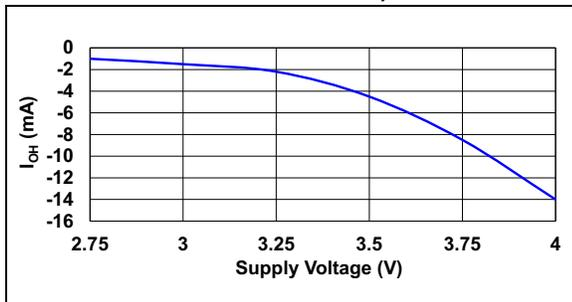
**FIGURE 1-8: OUTPUT SOURCE CURRENT VS. OUTPUT VOLTAGE (VCC = 3.3V, TA = +25°C)**
