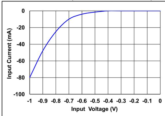
**FIGURE 1-12: INPUT CURRENT VS. INPUT VOLTAGE**
