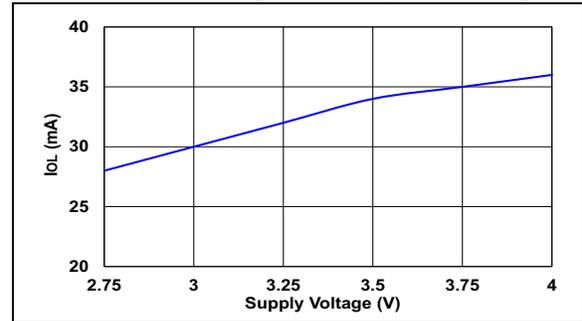
**FIGURE 1-10: OUTPUT SINK CURRENT VS. OUTPUT VOLTAGE (VCC = 3.3V, TA = 25°C)**
