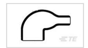
Body Orientation: Right Angle Molded Part Shape Code: 222
