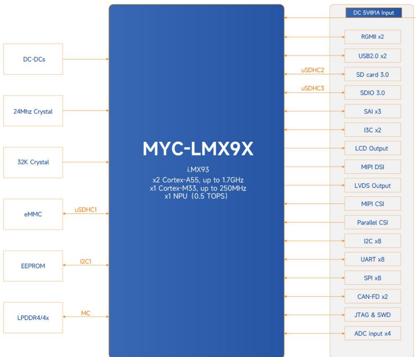
MYC-LMX9X Function Block Diagram
