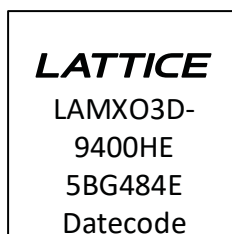
Figure 5.2. Top Markings for Automotive Grade Devices
