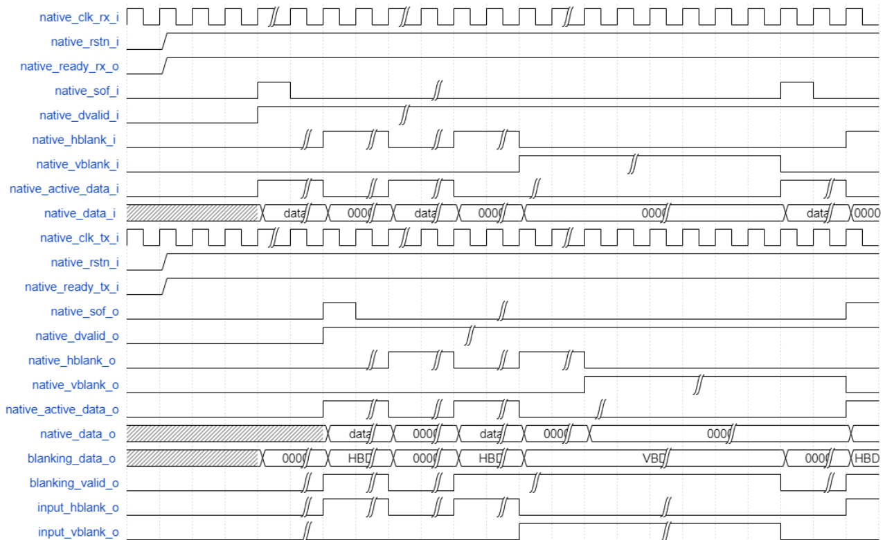
Figure 2.17. Native Input Video Timing Diagram with Blanking Related Signals
