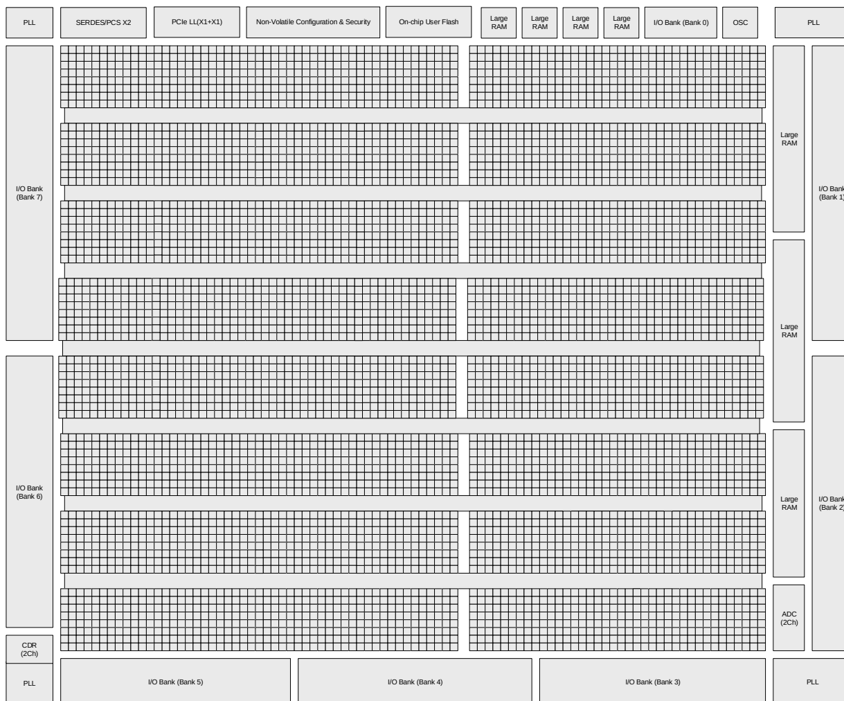
Figure 2.2. Simplified Block Diagram, MachXO5-NX-55T Device (Top Level)
