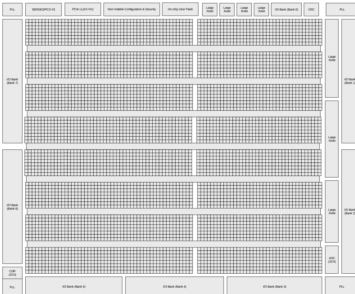
Figure 2.3. Simplified Block Diagram, MachXO5-NX-100T Device (Top Level)
