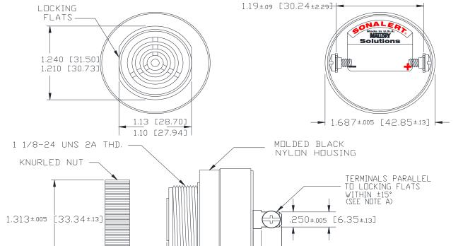
NOTE A: TERMINALS-.032 BRASS TIN PLATED, TAPPED FOR #6-32 SCREW. TWO #6-32 NICKEL PLATED BRASS SCREWS INCLUDED, WILL ACCEPT 1/4" QUICK CONNECT.
