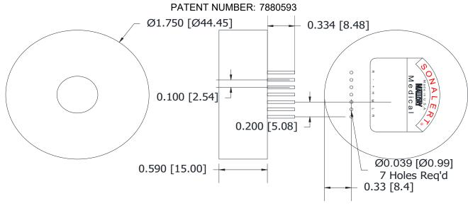
NOTE: Alarm functions at max dB. If a lower sound ouput is desired, add a 1/4 W resistor valued from  $27k\Omega$  down to a minimum  $100\Omega$  to achieve the desired sound level output. PIN OUT is R - + H M L R.
