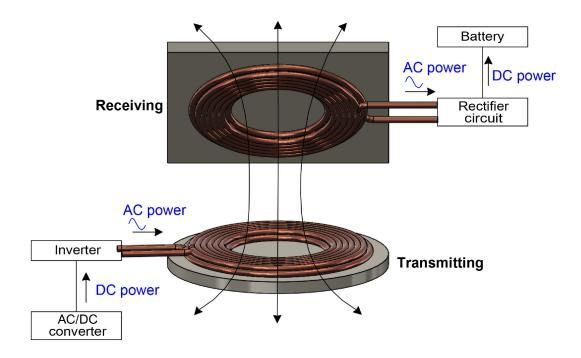
BEL | SERIES: WTSC | DESCRIPTION: WIRELESS CHARGING COIL (SINGLE WINDING)
