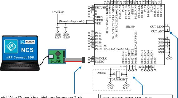
SWD (Serial Wire Debug) is a high performance 2-pin debug port that replaces JTAG. You can debug and program with J-link Lite. When using J-LINK Lite, it is convenient to mount a socket on the customer's main board. The socket will be "10-pin connector two rows of 1.27mm pitch (Ex: PSS-720153-05, Hirosugi instrument). J-Link Lite operates at 3.3 V. do not operate at 1.7 V, so please be careful.
